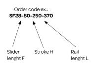
The SF ball-cage series are a linear rail with one or more sliders moving in a ball-cage, inside a longer rail. The components are the same as SR.
